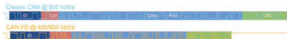
Figure 1: CAN FD allows higher bandwidth, even with slower arbitration
