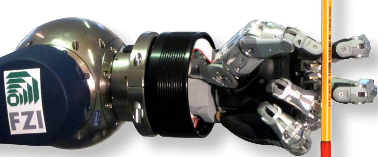
Figure 4: Human-sized servo-electric 5-finger hands from Schunk allow Hollie to grasp and manipulate objects (Photo: FZI)
