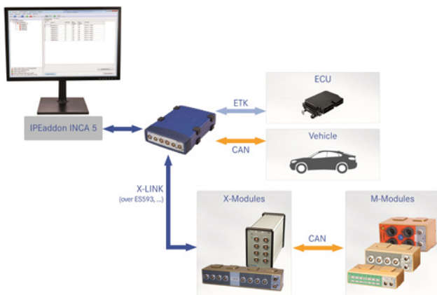
Figure 5: Application example of X-Link technology with control unit ES593 (Photo: Ipetronik)
